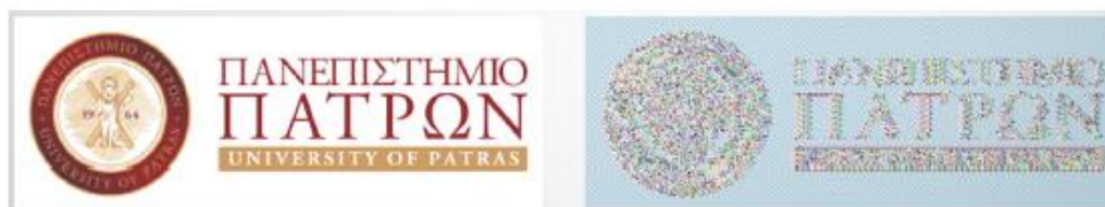
Fig. 9. (a) original image. (b) encrypted image using AES-ECB mode.
